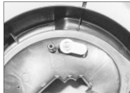
36.3b Air cleaner heat sensor viewed from inside air cleaner - OHC models
