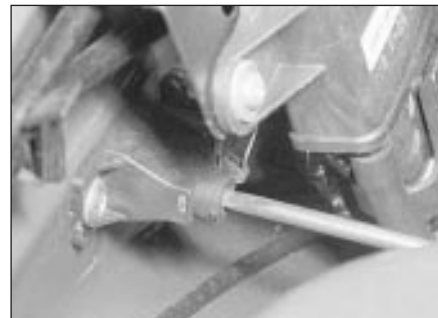
16.34b . . . to enable mixture adjustment - DOHC models
