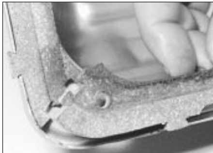
23.9a Camshaft cover gasket dovetails
