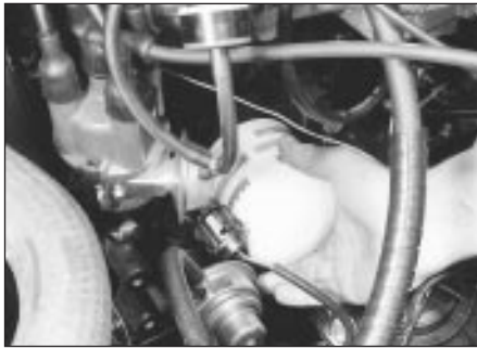
8.7 Unscrewing the oil filter
