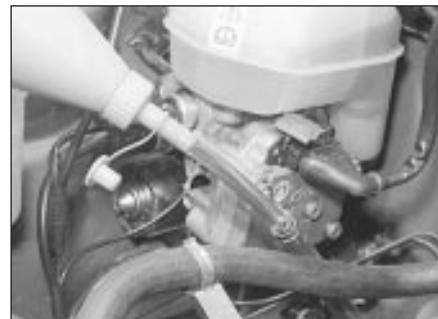
17.4 Topping-up the transmission fluid
