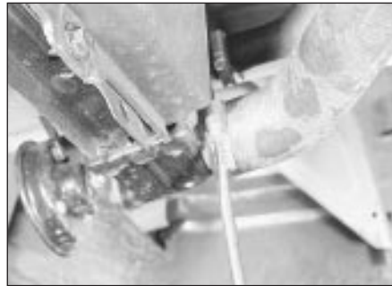
46.6a Disconnect the bottom hose from the radiator - early OHC models
