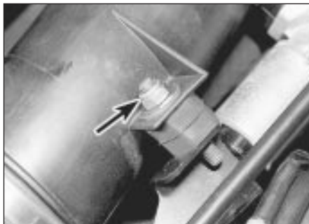
38.17 Air intake tube securing nut (arrowed)
