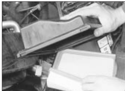
38.19 Lifting out the air cleaner element
