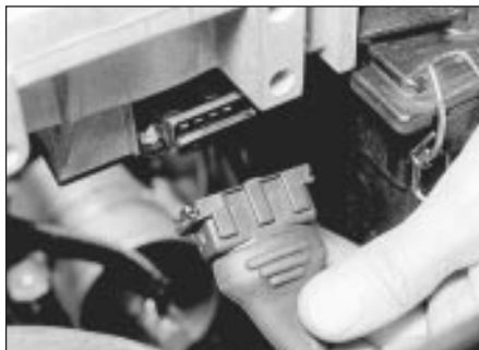
38.6 Disconnecting the airflow meter wiring plug
