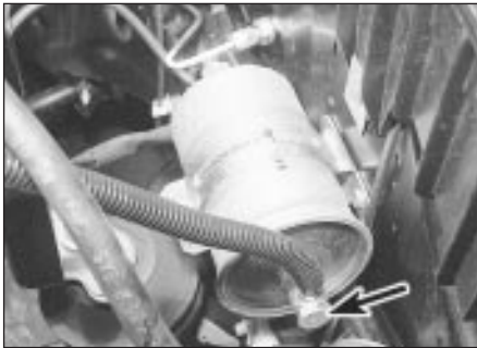
41.1 Fuel filter location - outlet union arrowed
