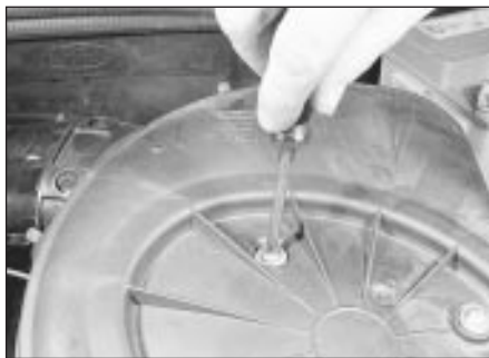
38.1 Remove the air cleaner cover screws . . .
