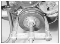
19.8 Using a puller to remove a pressed type crankshaft pulley
