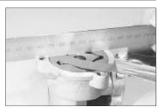
31.11 Checking the oil pump rotor endfloat
