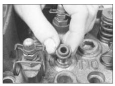
22.4 Removing a valve stem oil seal
