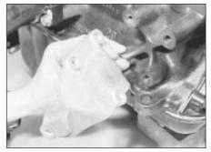
18.10b Removing the alternator mounting bracket
