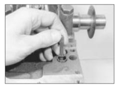
30.4 Withdrawing the oil pump driveshaft
