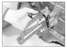
18.10a Removing the right-hand engine mounting bracket
