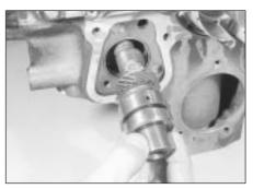
25.5b Withdraw the auxiliary shaft
