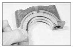
34.24 Fitting a thrustwasher to the centre main bearing cap
