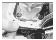
29.16 Locate the sump gasket end tabs beneath the rubber sealing strips
