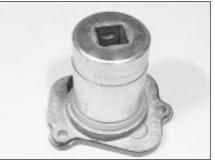
25.9b Using a socket to fit a new auxiliary shaft cover oil seal
