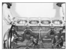
21.11 Fitting a new cylinder head gasket
