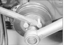
19.33 Holding a pressed type crankshaft pulley with two bolts and a lever while tightening the bolt
