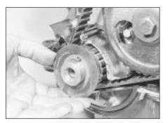
19.9 Removing the guide washer from the crankshaft
