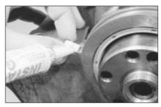
34.29 Fitting a sealing wedge to the rear main bearing cap
