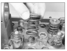
22.2b Removing a valve spring and cap
