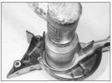
27.4 Using a socket to fit a new crankshaft front oil seal
