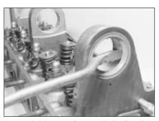
24.9 Prising out the camshaft oil seal
