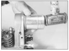
24.13 Fitting a new camshaft oil seal using a socket
