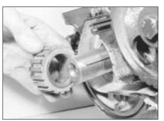
19.11 Removing the crankshaft sprocket
