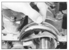
29.15b ... then fit the rubber sealing strips
