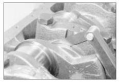
34.6 Checking crankshaft endfloat
