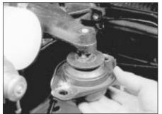
17.4 Withdrawing an engine mounting
