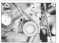
19.5 Timing belt tensioner bolts (arrowed) models from mid-1985
