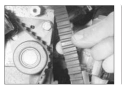
19.29 Twisting the timing belt to assess its tension
