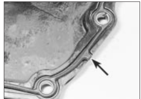
15.31 Lower timing chain cover rubber gasket in position. Ensure that lug on gasket engages with notch in cover (arrowed)
