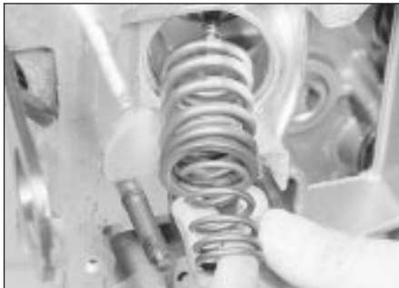
19.1 Withdrawing the double valve springs from the cylinder head
