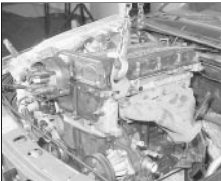
5.40 Lifting the engine from the vehicle
