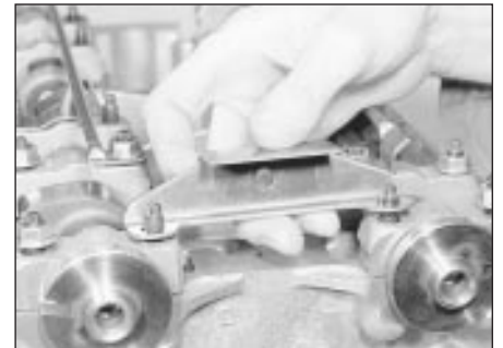
18.30c Fitting the timing chain guide plate
