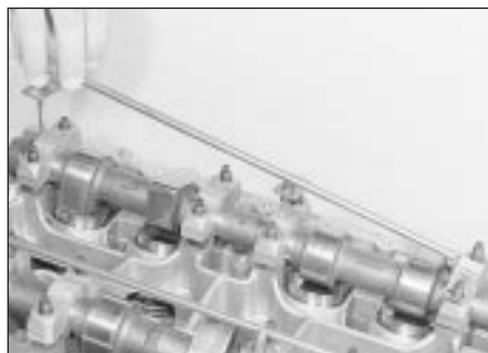
18.13 Lifting off a camshaft oil spray bar
