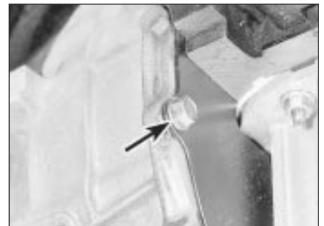
5.33 Engine adapter plate bolt (arrowed)
