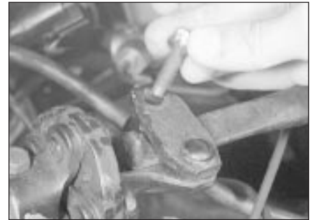
5.29 Removing the lower steering column clamp bolt
