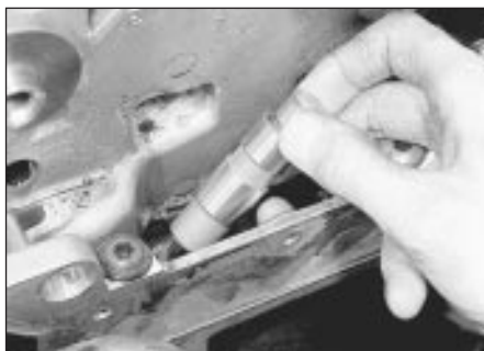
18.11 Lifting the chain tensioner plunger assembly from the cylinder head
