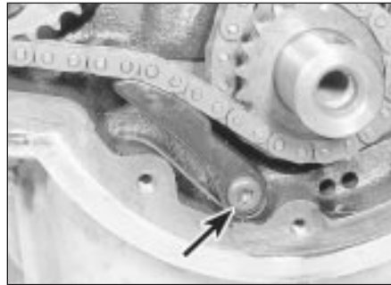
15.9 Oil pump chain tensioner securing screw (arrowed)
