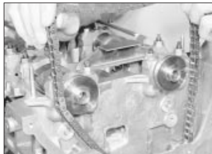
15.13 Withdrawing the timing chain through the top of the timing case
