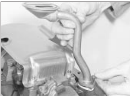
29.2 Removing the oil pick-up pipe
