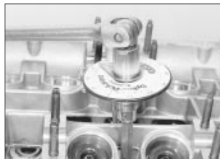
18.25b Tightening a cylinder head bolt using an angle gauge
