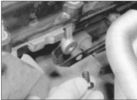
5.5 Removing the hose support bracket bolt from the cylinder head
