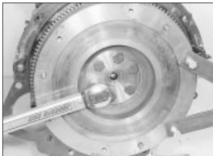
22.4 Improved tool used to hold flywheel when tightening securing bolts
