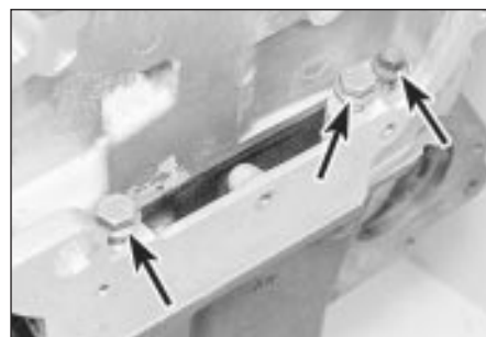
18.16 M8 cylinder head bolts (arrowed) located at front of cylinder head
