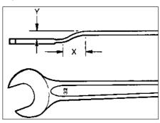
12.3 Modified spanner required for removing the thermo-viscous cooling fan
