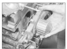
9.21 Withdraw the coolant pump
