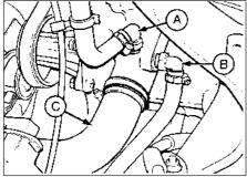
9.29 Coolant pump housing hose connections
