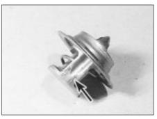
7.9 Thermostat flow direction markings (arrowed) cooling fan switch on the thermostat housing
