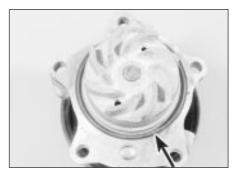
9.35 Coolant pump O-ring (arrowed)
