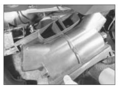
18.9 Withdrawing the heater
