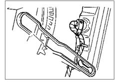
17.9 Heater control panel illumination bulb wiring loom correctly routed
