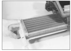
19.1b . . . and withdraw the heater matrix
