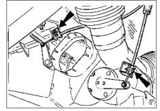
17.5 Heater control cable lower end fittings (arrowed)
