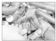
16.3b Disconnect the temperature gauge sender wiring - CVH
