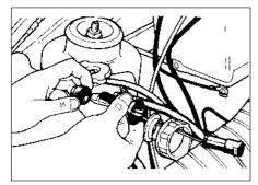
15.8a Removing the coolant level sensor from the expansion tank
