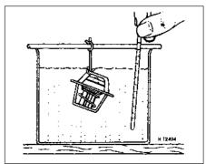
8.1 Testing the thermostat opening temperature
