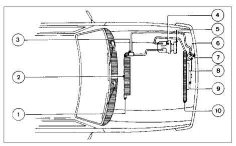
21.1 Layout of air conditioning system components
