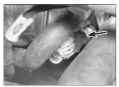
16.1 Temperature gauge sender location (arrowed)
