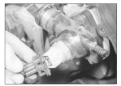
7.21 Disconnect the cooling fan switch wiring plug
