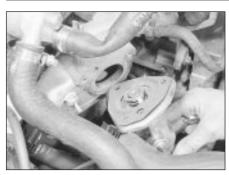
7.13 Removing the thermostat housing and gasket
