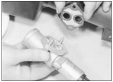
13.12 Withdrawing the idle speed control valve and gasket
