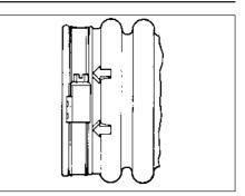
15.6 Air intake hose clip correctly aligned
