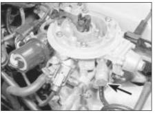
4.4 CFI unit fuel inlet union (arrowed)
