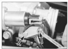
27.3 Unscrewing the throttle position sensor retaining bolts
