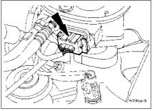
27.11b Throttle position sensor location (arrowed) on CFI unit - 1.8 litre (R6A) CVH
