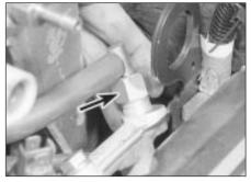
6.9 Fuel rail fuel feed union (arrowed)
