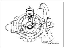
16.10 Align locating peg on injector with slot in CFI unit on refitting - 1.6 litre CVH
