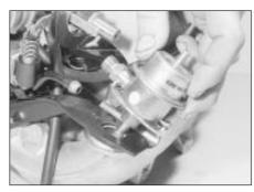
6.5 Withdrawing the fuel pressure regulator
