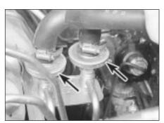
22.2 Pulse-air delivery check valves (arrowed)
