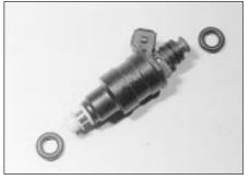
18.12 Fuel injector with seals removed
