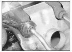
22.4 Unscrewing a pulse-air delivery tube union
