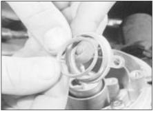
16.7 Removing the seal from the injector retaining collar
