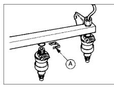
18.10 Fuel injector retaining clip (A)
