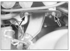
30.12 Lower inlet manifold bracket (arrowed)
