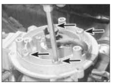
19.9 CFI unit securing bolts (arrowed) -1.6 litre CVH
