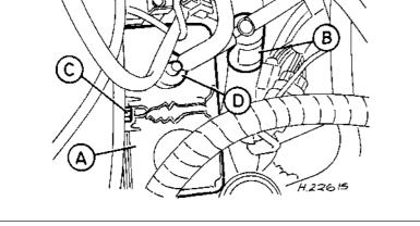
33.3 Carbon canister and purge solenoid locations - DOHC
