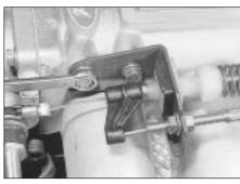
30.5 Unscrew the securing bolts and remove the throttle cable bracket
