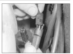
30.6 Disconnecting a fuel injection harness wiring plug
