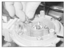
16.5a Removing an injector retaining collar securing bolt and locktab
