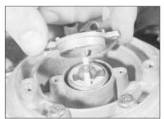
16.5b Removing the injector retaining collar
