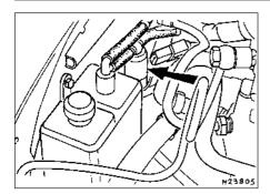
34.7 Carbon canister-purge solenoid location (arrowed) - 1.6/1.8 litre (R6A) CVH
