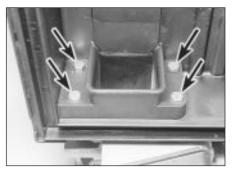
15.5 Airflow meter-to-air cleaner lid bolts (arrowed)
