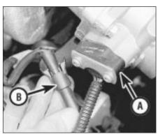
27.6 Throttle position sensor (A) and wiring plug (B)
