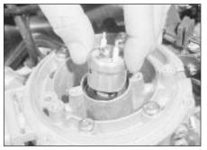
16.6 Withdrawing the fuel injector
