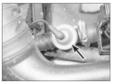
21.1 Pulse air system vacuum-operated air valve (arrowed)
