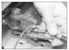
23.3 Disconnect the vacuum pipe connector from the solenoid
