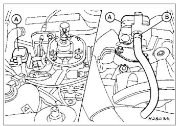
32.1 Exhaust pressure transducer attachments -1.8 litre (R6A) CVH
