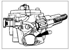
27.11a Throttle position sensor location (arrowed) on CFI unit - 1.6 litre CVH
