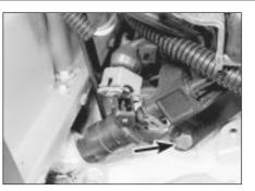
18.9a Fuel rail front securing bolt (arrowed) . . .
