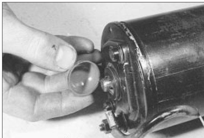
10.20a Remove the plastic cap from the end of the armature shaft . . .
