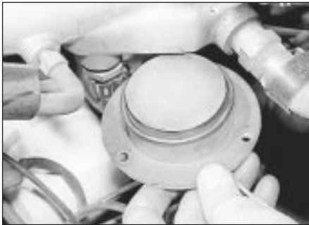
19.11 Removing inlet manifold heater - ESC II system
