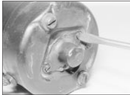
10.2 Remove the commutator end housing cap securing screws - Bosch long frame starter motor
