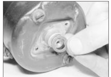
10.3b . . . and shims from the end of the armature shaft - Bosch long frame starter motor
