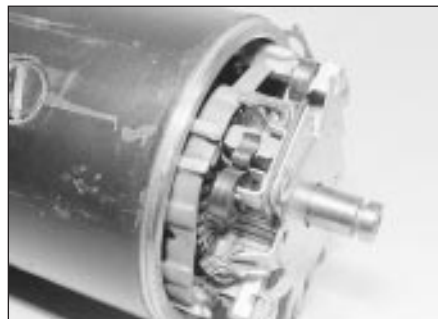
10.4b Commutator end housing removed to expose brush plate - Bosch long frame starter motor
