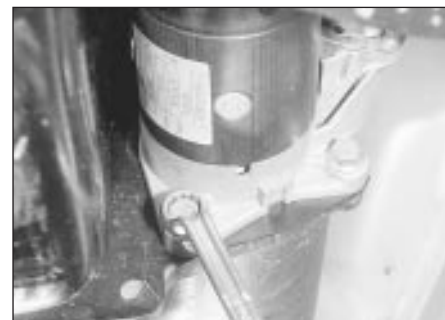
8.5 Unscrew the starter motor mounting bolts
