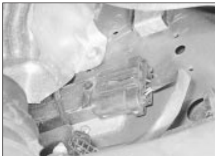
18.25 Ignition module location (arrowed)
