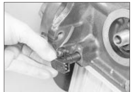
19.37 Removing the crankshaft speed/position sensor (engine removed)
