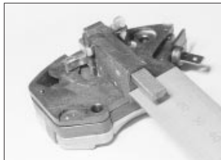
7.15 Compare the brush length with the figure given in the Specifications - Lucas A127 alternator
