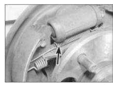
5.6a Top shoe return spring (arrowed)
