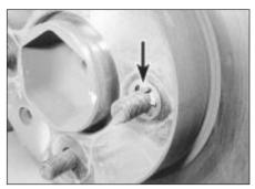
5.5a Brake drum retaining spire washer (arrowed)
