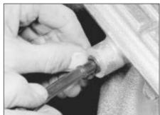
14.10 Disconnecting a later-type brake servo vacuum hose
