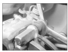
4.29 Unscrewing the forward caliper guide pin bolt
