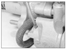
15.5a Remove the securing spring clip . . .
