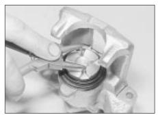
4.32 Retracting the piston using circlip pliers
