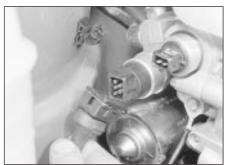
16.3c . . . and the pressure switch multi-plug - ABS
