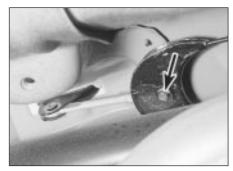
27.3 Handbrake equaliser securing circlip (arrowed) and pivot pin
