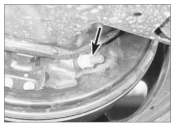
28.5 Plastic plunger (arrowed) in brake backplate
