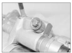
18.5 Hydraulic unit pump mounting bolt - ABS
