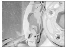
4.21a Later type front disc pad retaining clip
