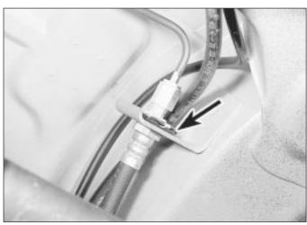
26.1 Flexible hose-to-rigid pipe union. U-shaped retaining clip arrowed
