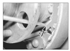
5.5c Drum removed showing screwdriver pressing on adjuster ratchet
