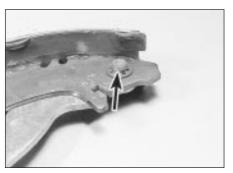
5.11 Handbrake lever-to-trailing shoe securing clip (arrowed)
