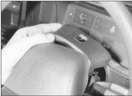
24.4a Remove the steering column upper shroud . . .
