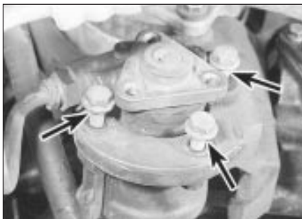
29.14a Unbolt the power steering pump pulley for access to the front pump securing bolts (arrowed)
