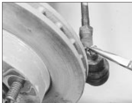
33.4 Extracting the split pin from the tie-rod balljoint castellated nut
