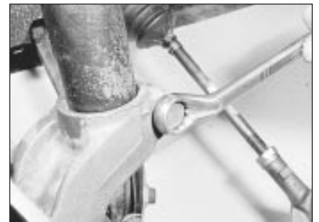
5.8 Unscrewing the hub carrier-to-strut pinch-bolt
