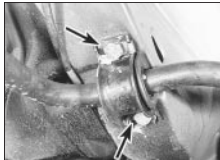
7.2a Bend back the locktabs (arrowed) . . .
