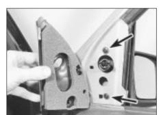
29.2 . . . and prise the mirror trim panel from the door to reveal the 3 mirror securing screws (2 arrowed)
