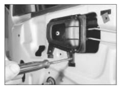
18.3a Remove the securing screws . . .
