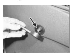
17.1b . . . then withdraw the window handle and bezel (arrowed)
