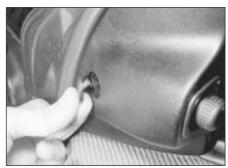
17.12a Prise the securing screw cover from the mirror control panel . . .
