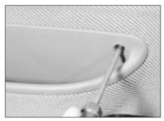
17.15b Trim panel securing screw at top edge of door pocket
