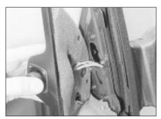
17.12b . . . and withdraw the mirror control panel
