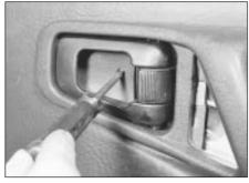
17.3a Remove the securing screw . . .
